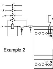
The thermostat is connected in series with the control circuit of the main contactor. When the temperature of the heatsink exceeds 90°C the main contactor will switch Off.
