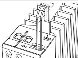
Optional thermal overload protection is possible by inserting a thermostat in a slot on the right hand side of the electronic contactor. Type number UP62
