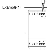
The thermostat can be connected in series with the control circuit of the electronic contactor. When the temperature of the heatsink exceeds 90°C the electronic contactor will switch Off.
